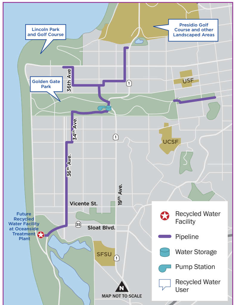
Project Facilities and Distribution System
