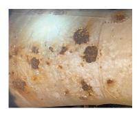
Corrosion Pitting at Manifold Piping
