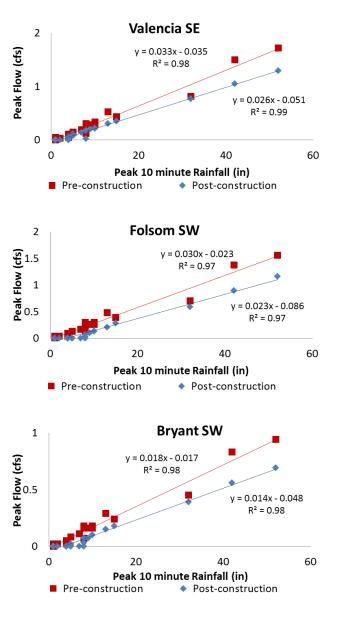
Figure 7. Estimated peak flow for each bioretention unit for pre- and post-construction conditions for corresponding peak 10 minute rainfall depths in each storm event.
