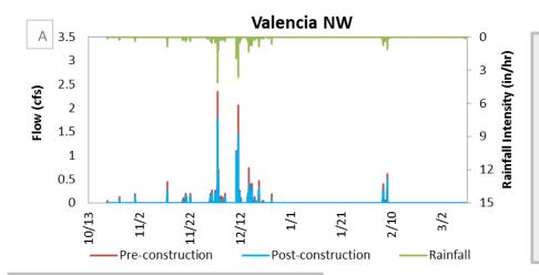
Flow reductions from Valencia NW were the lowest of the entire group due to the small ratio of GI area to DMA (0.5%). Nearly every storm resulted in outflows to the CSS. Nevertheless, this undersized unit still reduced estimated total flow volumes to the CSS by 31% over the course of the modeled season, and the estimated peak flow rate was reduced by 24% down to 1.77 cfs.
