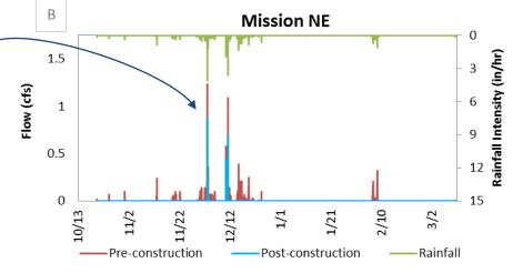
Figure 2. Modeled pre-construction versus post-construction flows and rainfall intensity at Cesar Chavez bioretention sites A) Valencia NW and B) Mission NE for the 2014-2015 rainy season.
