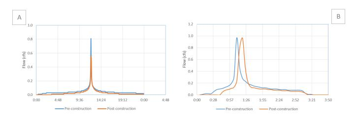
Figure 8. Estimated storm hydrograph for Valencia SE during the simulated: A) 1-year 24-hour storm, and B) 5-year 3-hour storm.
