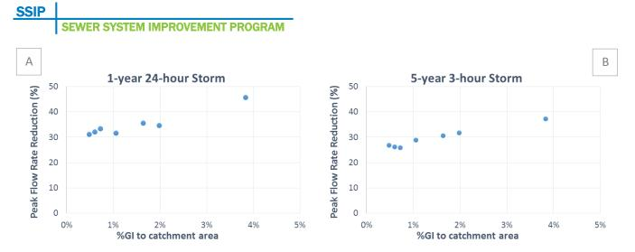
Figure 11. Estimated percentage of flow peak rate reduction in relation to ratio of GI area to DMA area: A) 1-year 24-hour storm, B) 5-year 3-hour storm.
