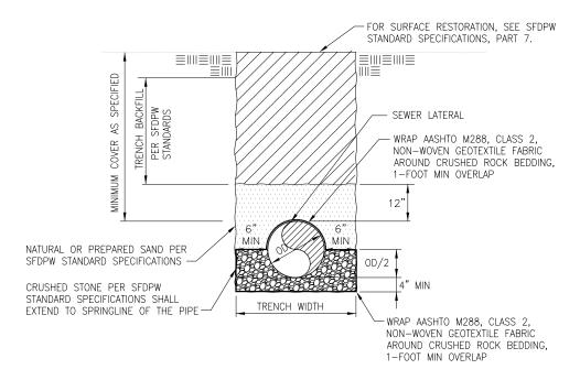
TRENCH DETAIL FOR RIGID PIPE NOT TO SCALE
