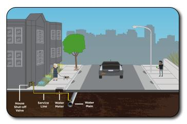
**Locate your service line**. Inspect where the line enters the home and check for leaks or listen for running water. A service line with a significant leak may cause standing water or ponding on the ground surface above the line, similar to a broken irrigation pipe. Lateral Insurance is available to all SFPUC homeowners – see <a href="https://www.awrusa.com/SanFrancisco">https://www.awrusa.com/SanFrancisco</a>
