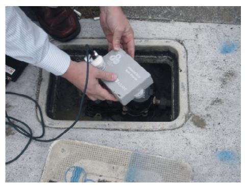
Top and bottom: Manual control override unit used to force more than one transmission every 15 minutes from MTU, to allow RF exposure measurements. Because the MTU is hermetically sealed, a magnetically-coupled control module is used to interface the MTU electronics.
