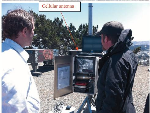
Top: DCU on roof of the Bernal Heights radio site building at 99 Moultrie Street. Bottom: DCU cabinet, with 838 MHz cellular and 462 MHz transmitters.
