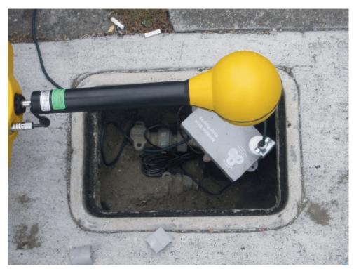
Top and bottom: Measurements at 8 inches (20 cm). The MTU has had the mounting brackets normally holding it to the bottom of the water vault concrete cover temporarily removed.
