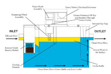
**Figure 3.** A typical design for an automatic grease removal device. Source: Thermaco, Inc.
