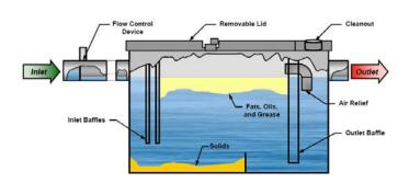
**Figure 2.** A typical design for a trap. Source: Bay Area Pollution Prevention Group
