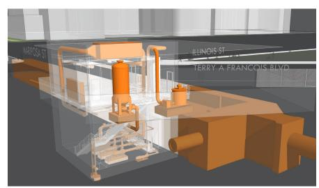
The Mariposa Pump Station upgrades include both above and below ground facilities.
